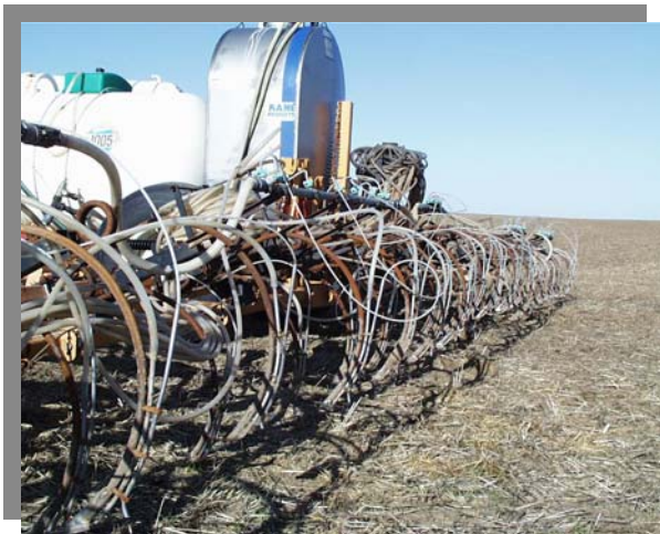
High disturbance shank fertilizer applicator.
