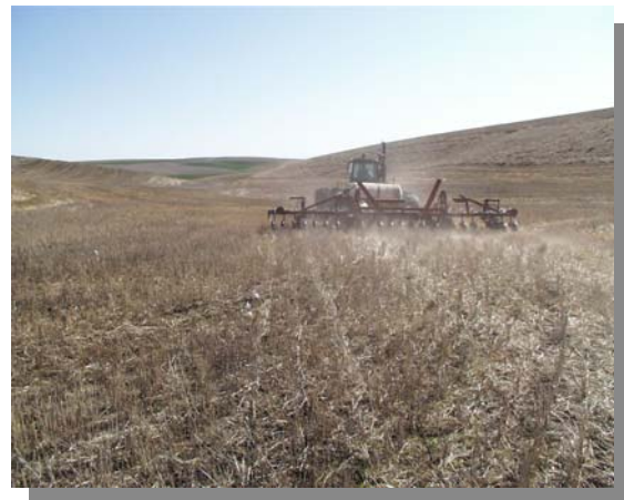
Low disturbance coulter fertilizer applicator.
