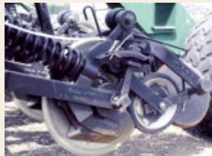
**Zenner's modified John Deere 1860 no-till air seeder (left) planting garbanzos into 70 bu/A durum wheat stubble. Close-up of the single-disk opener and packer wheel system (right).**
