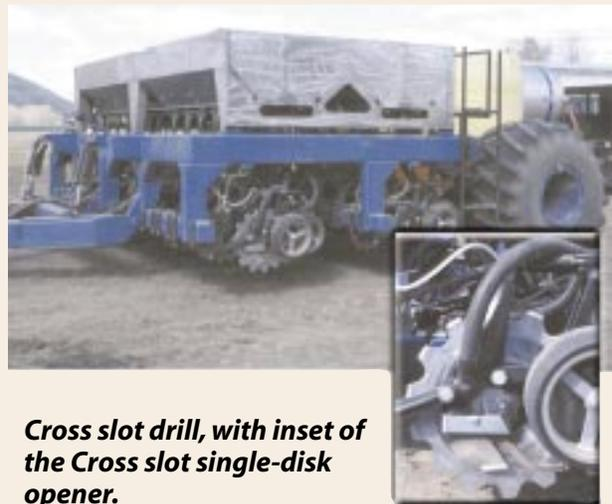
**Cross slot drill, with inset of the Cross slot single-disk opener.**
