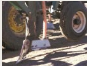
Ensleys' no-till drill seeding into harrowed chemical fallow, with close-ups of the drill and hoe-type opener.
