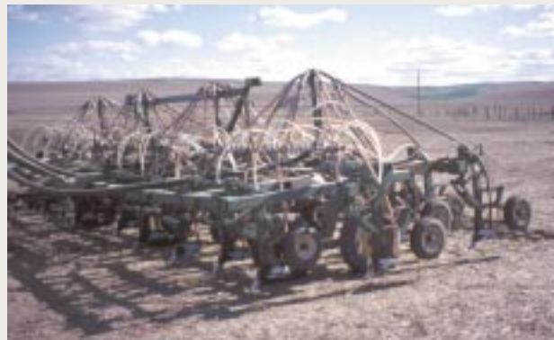
Ensleys' no-till drill seeding into harrowed chemical fallow, with close-ups of the drill and hoe-type opener.
