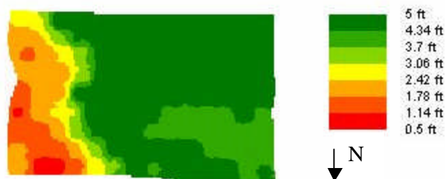
Figure 2. Depth to restricting layer or bedrock of the experiment site at the Sherman Experiment Station in Moro
