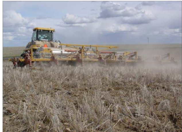
Primary spring tillage plus liquid aqua nitrogen injection with a V-sweep undercutter implement in the winter wheat - summer fallow region, 2005.
